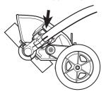
· Firmly tighten the screw.
