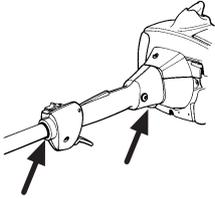
The machine's vibration damping system reduces the transfer of vibration between the engine unit/cutting equipment and the machine's handle unit.
