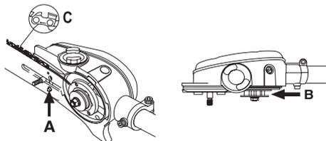
Tension the chain by turning the chain tensioning screw clockwise. Use a combination spanner or turn by hand. The chain should be tensioned until it fits snugly on the underside of the bar.
