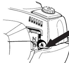
**Choke:** Set the throttle to the start position by moving the choke control to the choke position and then returning it to its original position.
