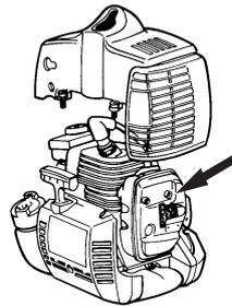
Some mufflers are equipped with a special spark arrestor screen. If your machine has this type of muffler, you should clean the screen at least once a week. This is best done with a wire brush.
