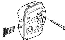
On mufflers without a catalytic converter the screen should be cleaned weekly, or replaced if necessary. On mufflers fitted with a catalytic converter the screen should be checked, and if necessary cleaned, monthly. **If the screen is damaged it should be replaced.**
