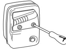
If the muffler on your machine is fitted with a spark arrestor screen this must be cleaned regularly. A blocked screen will cause the engine to overheat and may lead to serious damage.
