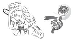
IMPORTANT! In order to maintain operation of the centrifugal cleaning system it must be regularly maintained. Clean the air intake to the starter, the fins on the flywheel, the space around the flywheel, inlet pipe and carburetor compartment.
