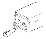
Some mufflers are equipped with a special spark arrestor screen. If your machine has this type of muffler, you should clean the screen at least once a week. This is best done with a wire brush. A blocked screen will cause the engine to overheat and may lead to serious damage.
