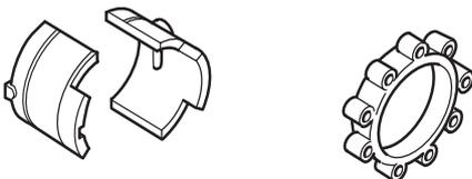
Regularly check the vibration damping units for cracks or deformation. Check that the vibration damping element is undamaged and securely attached.
