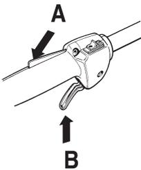
Make sure the throttle control is locked at the idle setting when the throttle lockout is released.
