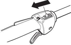
**Choke:** Put the choke in working position.
