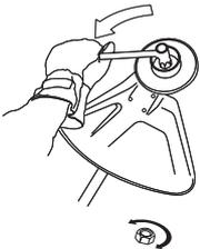
The nylon lining inside the locking nut must not be so worn that you can turn it by hand. The lining should offer a resistance of at least 1.5 Nm. The nut should be replaced after it has been put on approx. 10 times.
