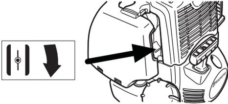
**Primer bulb:** Press the air purge repeatedly until fuel begins to fill the bulb. The bulb need not be completely filled.
