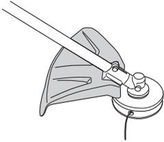
Check that the guard is undamaged and not cracked. Replace the guard if it has been exposed to impact or is cracked.
