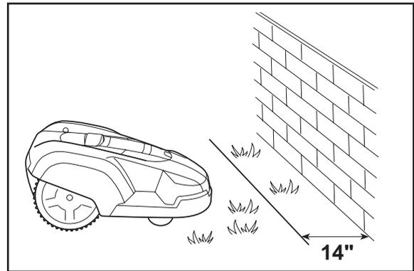
If the working area borders against a small ditch, for example, a flower bed or a small elevation, e.g. a low verge (1" - 2"), the boundary wire should be laid 12" inside the working area. This prevents the wheels from driving into the ditch or up onto the verge.
