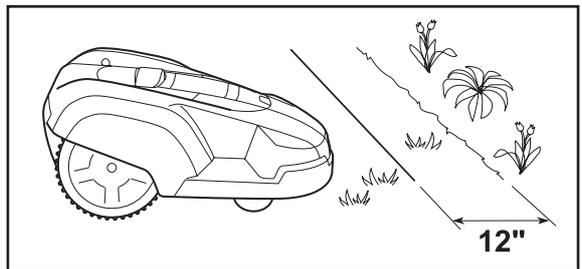
If the working area borders against a flat path or the like that lies level with the lawn, it is possible to allow Automower to run a little over the path. The boundary wire should then be laid 4" from the edge of the path.
