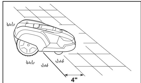
When the working area is divided by a flat slab path that is level with the lawn, it is possible to allow Automower to run over the path. It can be an advantage to lay the boundary wire under the slabs. The boundary wire can also be laid in the joint between the slabs.
