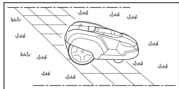
If the working area borders against, for example, pools of water the boundary wire should be supplemented with a fence or the like. The height must then be at least 6". This will prevent Automower, under any circumstances, coming outside of the working area.
