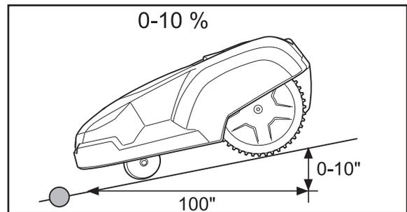
The boundary wire should not be laid across a slope that is steeper than 10 %. There is a risk of Automower finding it difficult to turn, and being unable to move. The risk is at its greatest in damp weather conditions, as the wheels can slip on the wet grass.
