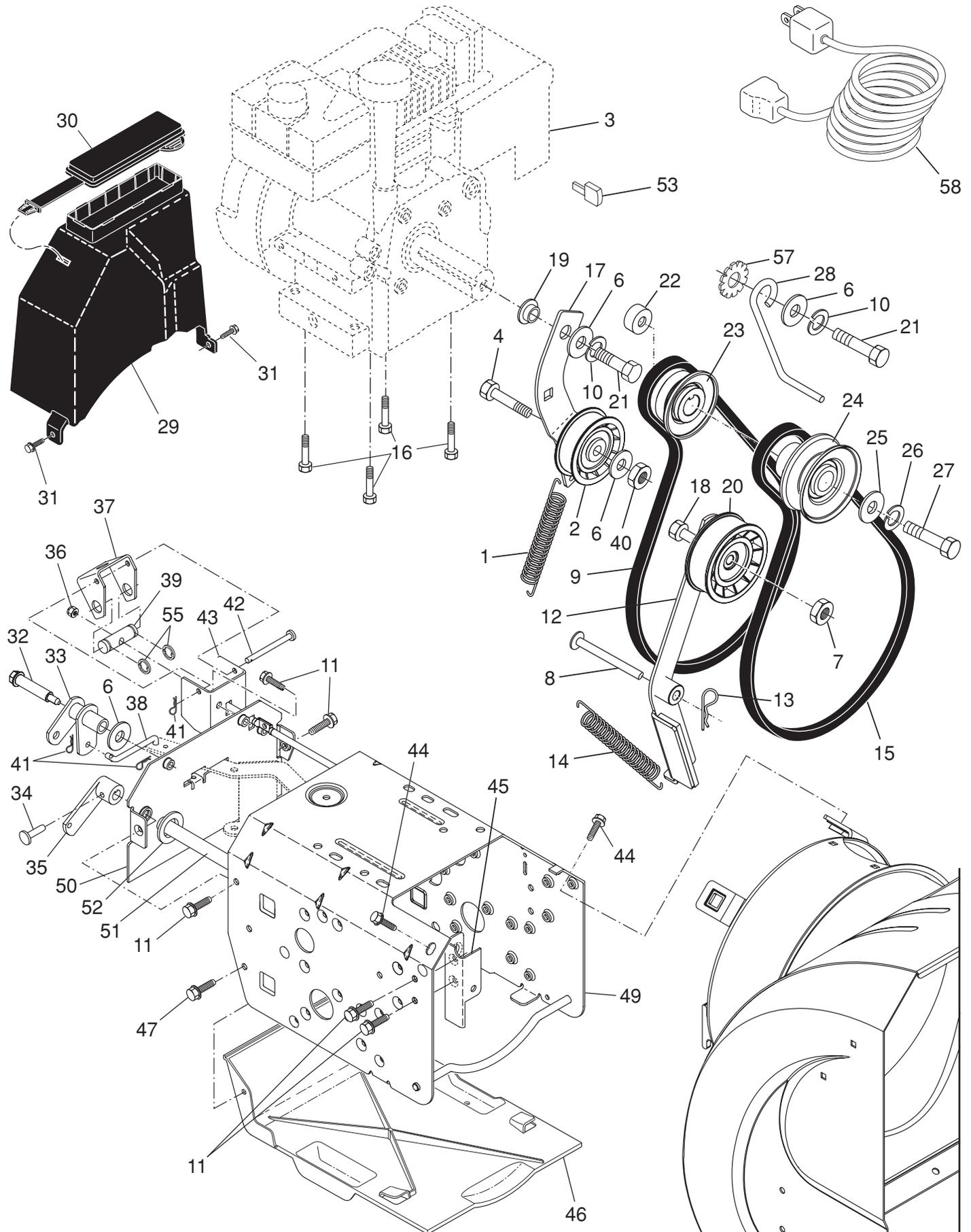
**REPAIR PARTS****CHASSIS / ENGINE / PULLEYS****SNOW THROWER - MODEL NO. 924SBE (96193002201), PRODUCT NO. 961 93 00-22**
