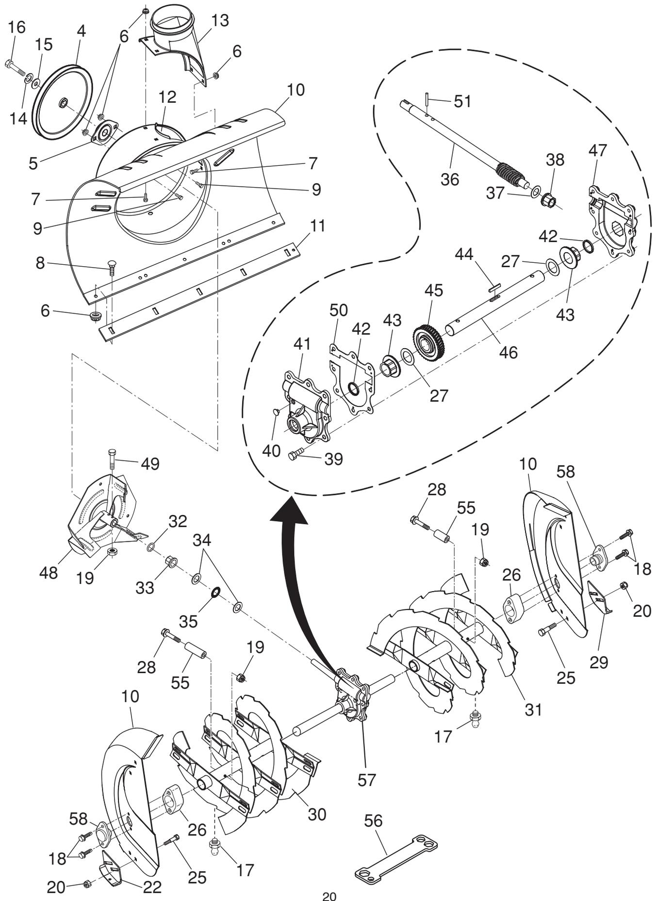
**REPAIR PARTS****AUGER HOUSING / IMPELLER ASSEMBLY****SNOW THROWER - MODEL NO. 924SBE (96193002201), PRODUCT NO. 961 93 00-22**
