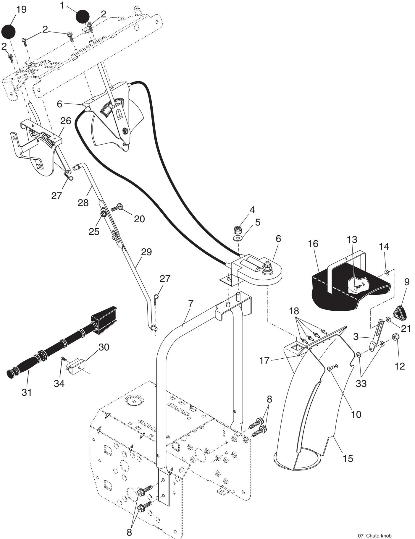
**REPAIR PARTS****CONTROL PANEL / DISCHARGE CHUTE****SNOW THROWER - MODEL NO. 924SBE (96193002201), PRODUCT NO. 961 93 00-22**
