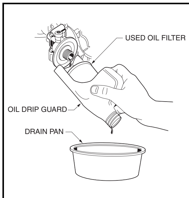
Figure 20 Remove Engine Oil Filter
