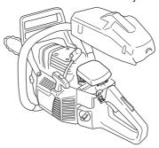
The filter can be cleaned more thoroughly by washing it in water and detergent.
