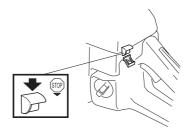
The engine is stopped by pushing the stop switch to the stop position.
