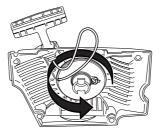
Undo the screw in the centre of the pulley and remove the pulley. Insert and fasten a new starter cord to the pulley. Wind approx. 3 turns of the starter cord onto the pulley. Connect the pulley to the recoil spring so that the end of the spring engages in the pulley. Fit the screw in the center of the pulley. Insert the starter cord through the hole in the starter housing and the starter handle. Make a secure knot in the end of the starter cord.
