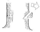
The directional cuts should run 1/4 of the diameter through the trunk and the angle between the top cut and bottom cut should be 45°.
