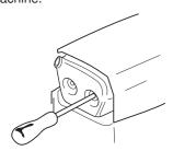
Some mufflers are equipped with a special spark arrestor screen. If your machine has this type of muffler, you should clean the screen at least once a week. This is best done with a wire brush. A blocked screen will cause the engine to overheat and may lead to serious damage.
