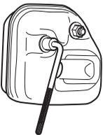
If the muffler on your machine is fitted with a spark arrestor screen this must be cleaned regularly. A blocked screen will
