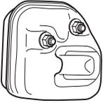
In countries that have a warm and dry climate there is a significant risk of fire. We therefore fit certain mufflers with a spark arrestor screen. Check whether the muffler on your machine is fitted with this kind of screen.
