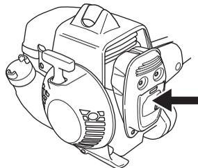
Some mufflers are equipped with a special spark arrester screen. If your machine has this type of muffler, you should clean the screen at least once a week. This is best done with a wire brush. On mufflers without a catalytic converter the screen should be cleaned weekly, or replaced if necessary. On mufflers fitted with a catalytic converter the screen should be checked, and if necessary cleaned, monthly. **If the screen is damaged it should be replaced.** If the screen is
