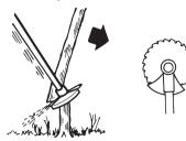
To fell a tree forwards, the bottom of the tree should be pulled backwards. Pull the blade backwards with a quick, firm movement.
