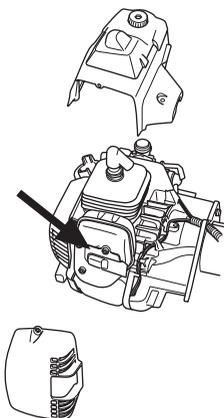
Some mufflers are equipped with a special spark arrester screen. If your machine has this type of muffler, you should clean the screen at least once a week. This is best done with a wire brush.
