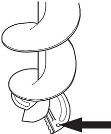
When the blade is manufactured it is sharpened using an advanced method. This means that the blade cannot be re-sharpened using conventional methods. Worn blades must be replaced with new ones to ensure your machine works satisfactorily.
