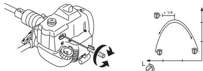
**CAUTION!** If the blades move while the engine is idling the T screw should be turned anti-clockwise until they stop.
