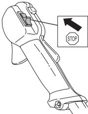
**CAUTION!** The stop switch automatically returns to the start position. In order to prevent unintentional starting, the spark plug cap must be removed from the spark plug when assembling, checking and/or performing maintenance.
