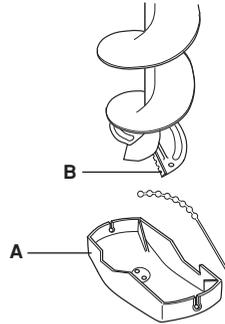
Regularly check that the transport guard is not damaged. Replace the transport guard if it is damaged.
