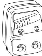
In countries that have a warm and dry climate there is a significant risk of fire. We therefore fit certain mufflers with a spark arrestor screen. Check whether the muffler on your machine is fitted with this kind of screen.
