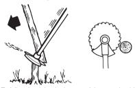
To fell to the right, the bottom of the tree should be pushed to the left. Tilt the blade and bring it diagonally up to the right. Cut with the area of the blade between 3 o'clock and 5 o'clock so that the direction of rotation of the blade pushes the bottom of the tree to the left.
