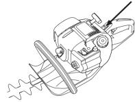
**CAUTION!** The stop switch automatically returns to the start position. In order to prevent unintentional starting, the spark plug cap must be removed from the spark plug when assembling, checking and/or performing maintenance.
