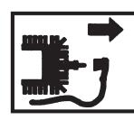
Switch off the engine by releasing the engine brake handle before carrying out any checks or maintenance.
