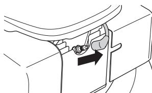
Do not fill too much petrol. Leave about 35 mm under the filler cap so that the fuel can expand.
