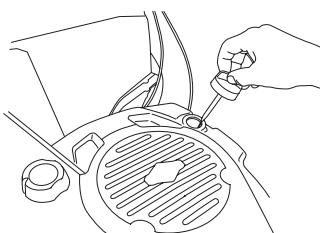
The oil filler cap must be completely screwed down to give a correct picture of the oil level.
