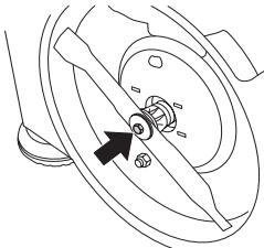
If the cutter or cutter bracket need to be changed you must replace the cutter bolt, washer and cup spring at the same time.
