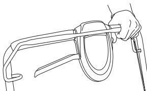
Grip the starter handle, slowly pull out the cord with your right hand until you feel some resistance (the starter pawls grip), now quickly and powerfully pull the cord. **Never twist the starter cord around your hand.**
