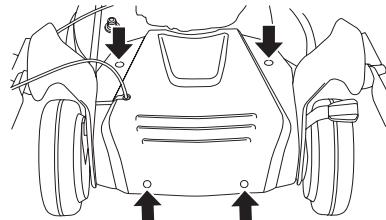
The cutting cover is designed to reduce vibration and to reduce the risk of cuts. Make sure the cutting cover is not damaged and that there are no visible defects such as cracks.
