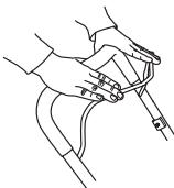
The brake handle must never be permanently anchored in handle when the machine is running.
