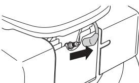
Unscrew the oil filler cap and check the oil level on the dipstick fitted to the cover.
