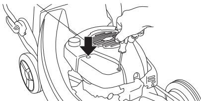
Remove the air filter and check that it is undamaged. Replace with a new air filter if you believe it to be defective.
