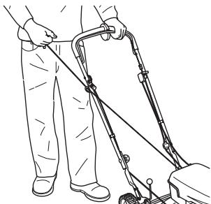
**CAUTION!** Do not pull the starter cord all the way out and do not let go of the starter handle when the cord is fully extended. This can damage the machine.
