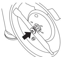
The washer and cup spring should always be replaced when changing the cutter or cutter bracket.
