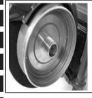
Mount the Ring Beveler assembly onto the hub shaft.
