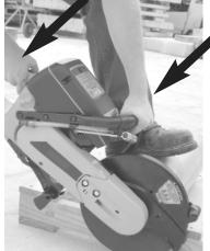
HOLD MACHINE ONLY at front and rear handles, as shown in the photo to the left.
