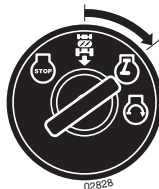
Engine "ON" Position (Normal Operating)
