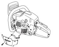
CAUTION! If the special winterising kit has been fitted or any measures have been taken to increase the temperature these changes must be reversed before the machine is used in normal temperature conditions. Otherwise there is a risk of overheating, resulting in severe damage to the engine.
