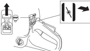
**Startgass:** Kombinert choke/startgass-stilling oppnås når hendelen stilles i chokesetting.
