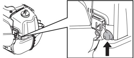
**Choke:** Set the choke control in the choke position.
