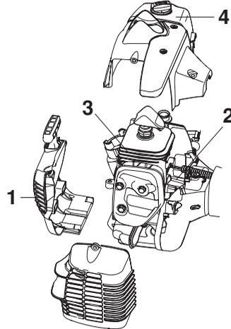
The cooling system consists of:
