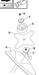
Hook the blade guard/combination guard (A) onto the fitting on the shaft and secure with the bolt.
