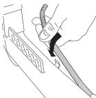
Put on the harness and hang the machine from the support hook. Now make a final adjustment so that the machine is in a comfortable working position when it hangs from the harness. Tighten the knob.
