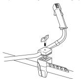
Put on the harness and hang the machine from the support hook. Now make a final adjustment so that
