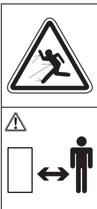
Do not remain within the broom unit's operating range, which is equivalent to a radius of 10 metres.
