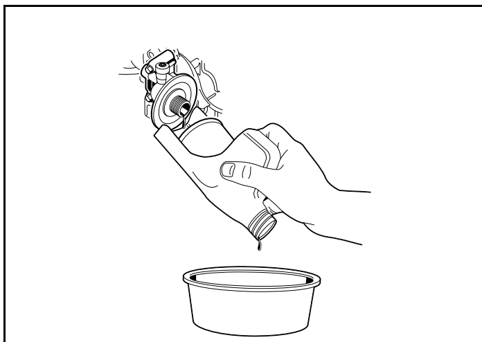
Figure 28 Remove Engine Oil Filter
