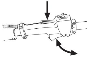
See instructions under the heading Start. Start the machine and apply full throttle. Release the throttle and check that the cutting attachment stops and remains at a standstill. If the cutting attachment rotates with the throttle in the idle position then the carburettor idle setting must be checked. See instructions under the heading Maintenance.
