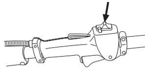
Start the engine and make sure the engine stops when you move the stop switch to the stop setting.
