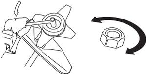
The nylon lining inside the locking nut must not be so worn that you can turn it by hand. The lining should offer a resistance of at least 1.5 Nm. The nut should be replaced after it has been put on approx. 10 times.
