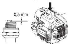
**CAUTION!** Always use the recommended spark plug type! Use of the wrong spark plug can damage the piston/cylinder.
