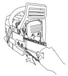
The chain is correctly tensioned when it does not sag from the underside of the bar, but can still be turned easily by hand. Hold up the bar tip and tighten the bar nuts with the combination spanner.
