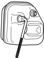
If the muffler on your machine is fitted with a spark arrestor screen this must be cleaned regularly. A blocked
