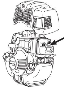
The muffler on your machine is equipped with a spark arrestor screen, this should be cleaned regularly. A blocked screen will cause the engine to overheat and may lead to serious damage.
