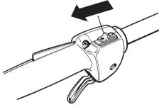
**Choke:** Put the choke in working position.
