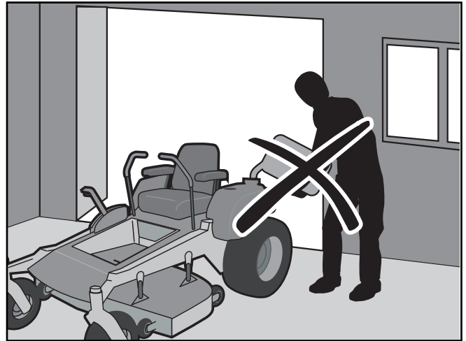
Never fill the fuel tank indoors
