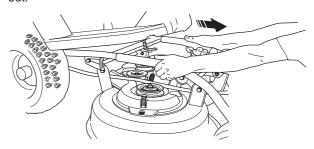
9 Lift off the deck and lean it against the machine or a wall.
