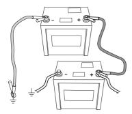
Connect each end of the red cable to the POSITIVE pole
