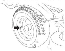
**IMPORTANT INFORMATION** Different tyre pressures on the front tyres will result in the blades cutting the grass at different heights.
