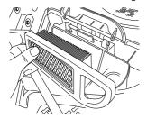
5 Replace the air filter cartridge, if clogged with dirt.
