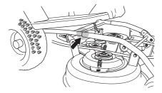
3 Push the cutting deck in and make sure the guide bolts fit into the grooves on the deck frame, one on each side.
