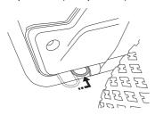
2 Lift up the cutting unit by pulling the lever backwards to its locked position.
