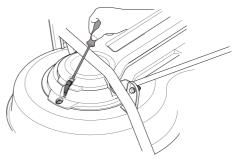
6 Loosen the spring on the drive belt's belt idler by loosening the handle.
