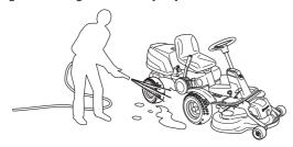
Oily dirt can be removed using a cold degreasing agent. Spray on a thin layer.
