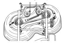
7 Tension the belt with the belt adjuster.
