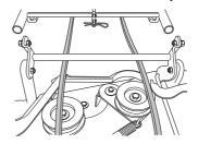
2 Fit the cutting deck's pipe together with the deck frame's pipe.
