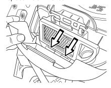
10 Pull the handle outwards. Secure the handle in the air filter cover and close the cover by pressing it inwards.
