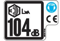
Noise emission to surroundings in accordance with the directive of the European Community. The machine's emission is indicated in the TECHNICAL DATA chapter and on the decal.
