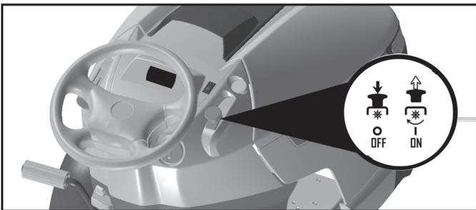
(☒) ATTACHMENT CLUTCH SWITCH "DISENGAGED"
