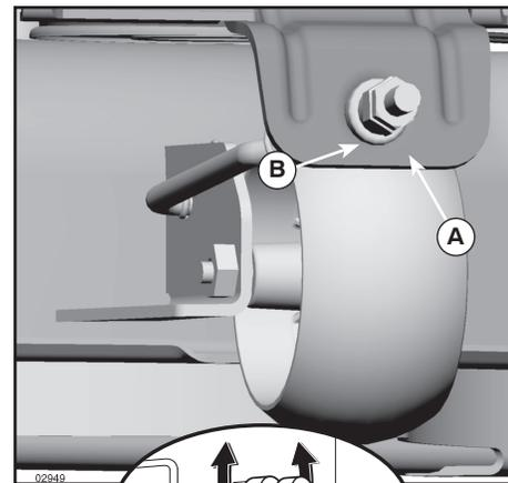
Tighten adjust nut B to raise mower
