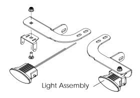
2. Using the kit wire tie, secure the light wiring to the light brackets through the rear bracket holes. Plug wiring into kit pigtail.
