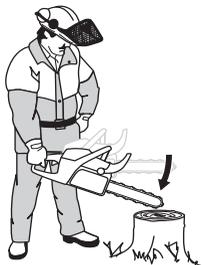
When the bar hits the stump the brake should be applied.
