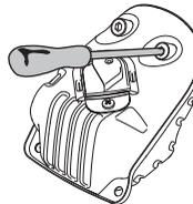
Some mufflers are equipped with a special spark arrester screen. If your machine has this type of muffler, you should clean the screen at least once a week. This is best done with a wire brush. A blocked screen will cause the engine to overheat and may lead to serious damage.
