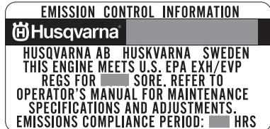
The Emissions Compliance Period referred to on the Emission Compliance label indicates the number of operating hours for which the engine has been shown to meet Federal emissions requirements.
