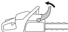
Remove the bar nuts and remove the clutch cover (chain brake). Take off the transportation ring (A).
