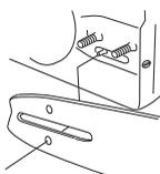
Tension the chain by turning the chain tensioning screw clockwise using the combination spanner. The chain should be tensioned until it does not sag from the underside of the bar. See instructions under the heading Tensioning the chain.
