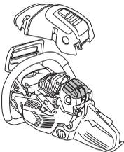
The filter can be cleaned more thoroughly by washing it in water and detergent.
