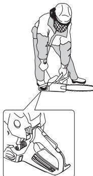
As the chain brake is still activated the engine must return to idling speed as soon as possible by disengaging the throttle latch in order to avoid unnecessary wear on the clutch assembly.
