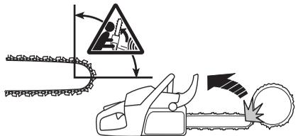
Cutting with the bottom edge of the bar, i.e. from the top of the object downwards, is known as cutting with a pulling chain. In this case the chain saw pulls itself towards the tree and the front edge of the chain saw body rests naturally on the trunk when cutting. Cutting with a pulling chain gives the operator better control
