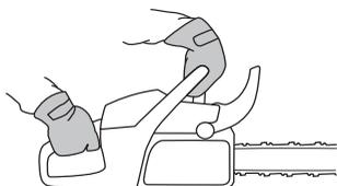
Apply full throttle and activate the chain brake by tilting your left wrist forward onto the front hand guard. Do not let go of the front handle. **The chain should stop immediately.**
