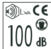
Noise emissions to the surroundings in accordance with the European Union's directive. The machine's emission is stated in the chapter TECHNICAL DATA and on the decals. Only machines for European market
