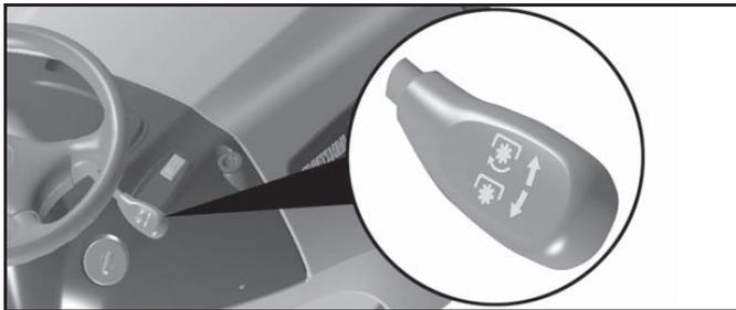
(☒) ATTACHMENT CLUTCH LEVER “DISENGAGED”
