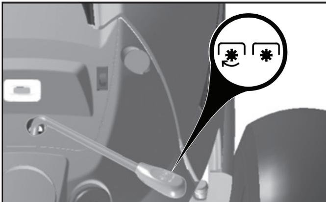
(☞) ATTACHMENT CLUTCH LEVER "DISENGAGED"
