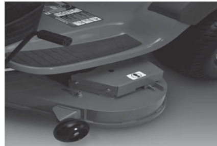
Fabricated Deck Shell Example Below
