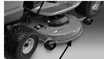
Armor Protected Stamped Deck Shell Reinforced area
