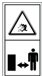
Do not stand in the machine's working area. Make sure there are no stones, twigs and other rubbish on the lawn. This type of object can be thrown by the machine and cause personal injury or damage to the machine. Avoid driving over gravel paths, etc.
