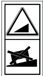
Never use the machine if downwards on slopes with an incline is greater than 10 degrees.
