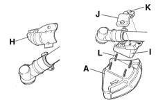
Remove the mounting plate (H). Fit the adapter (I) and bracket (J) with the two screws (K) as shown. Fit the blade guard (A) to the adapter using the 4 screws (L) as shown.
