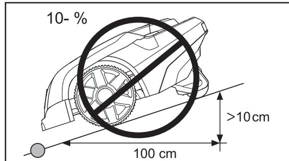
However, the boundary wire can be laid across a slope steeper than 10 % when there is an obstacle that Automower® can be permitted to collide with, for example, a fence or a dense hedge.
