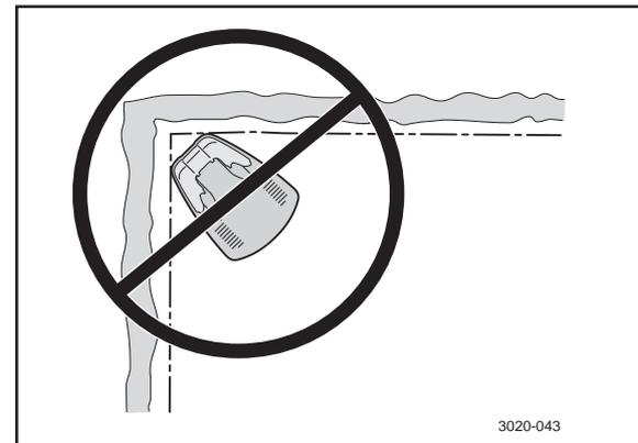
The charging station must be positioned on relatively level ground. The front end of the charging station must be a maximum of 1.5" (3 cm) higher than the back end. The front end of the charging station must never be lower than the back end.
