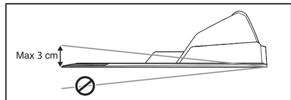
The charging station must not be positioned so that its plate bends.
