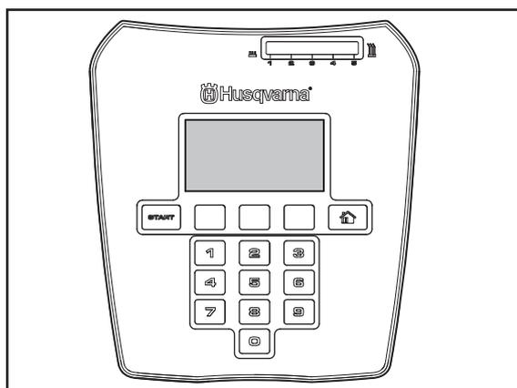
When the stop button has been pressed and the cover is opened, the operation window appears to display the clock, selected operating mode, number of mowing hours, battery status and timer setting.
