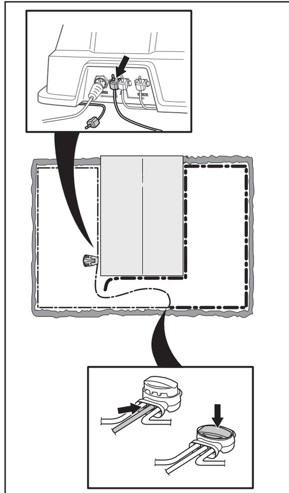
In that case, move the connection for the new wire closer to the disconnected end (roughly at the middle of the suspect wire section) and check again if the indicator light is green or flashes yellow.
