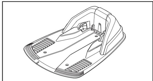
2. Check that the boundary wire connections to the charging station are properly connected and not damaged. Check that the indicator light in the charging station is still flashing blue.
