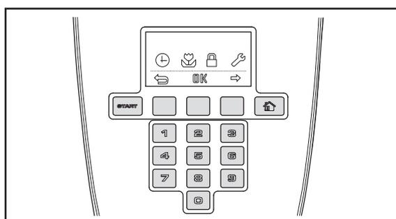
The keypad consists of four groups of buttons: operation selection button, multi-choice buttons, numbers and start button.
