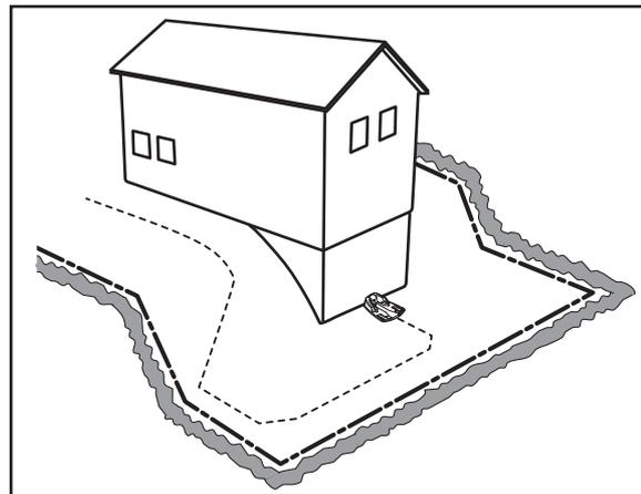
Avoid laying the wire at sharp angles. This can make it difficult for the mower to follow the guide wire.
