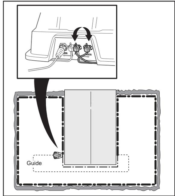
b) Put A1 and Guide back in their original positions. Then switch A2 and Guide. If the indicator light flashes yellow, then the break is somewhere on the boundary wire between A2 and the point where the guide wire is connected to the boundary wire (thick black line in the illustration).
