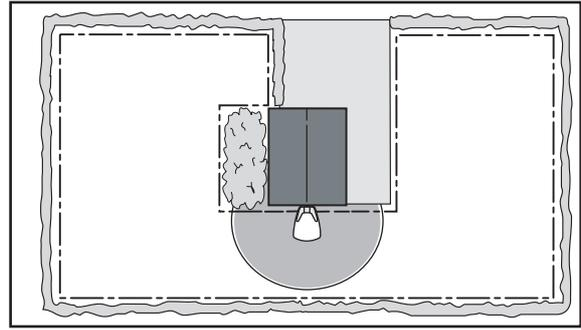
Do not put the charging station in confined spaces in the working area. There must be a straight boundary wire, at least 5 feet (1.5 metres) long, to the right and left of the charging station. The wire must be laid straight out from the rear end of the charging station. Any other locations can mean that the lawn mower enters the charging station sideways and will have difficulty docking.
