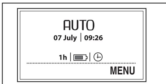
The battery status shows the remaining battery charge.
