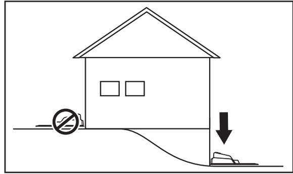
The charging station should not be placed on an island as this limits the laying of the guide wire in an optimal way. If the charging station has to be installed on an island, the guide wire also has to be connected to the island. See the picture opposite. Read more about islands in chapter 3.4 *Installation of the boundary wire*.
