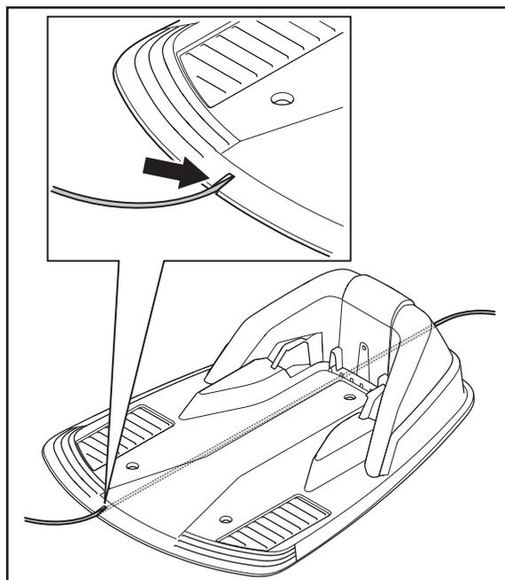
2. Fit the connector to the guide wire in the same way as for the boundary wire in 3.5 *Connecting the boundary wire*. Connect it to the contact pin on the charging station that is labelled "guide".
