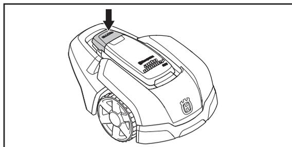
The control panel consists of a display and a keypad. All information is shown on the display and all input is done using the buttons.
