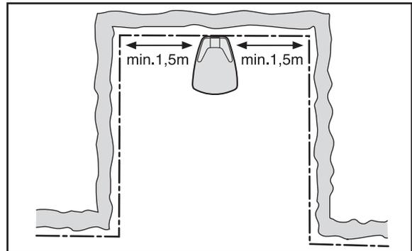
Do not put the charging station in a corner in the working area.
