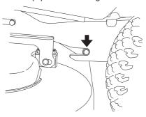
8 Fit the drive belt around the drive wheels of the cutting unit. Make sure the belt is placed on the correct side of the belt tensioner wheel.
