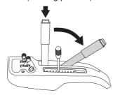
The lever can also be used to temporarily regulate the cutting height, e.g. for a small mound in the lawn.
