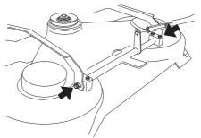
7 Remove the screws on the cutting cover. Lift the unit frame and remove the cutting unit cover.
