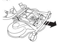
9 Lift the unit until it stops and a clicking sound is heard. The unit locks automatically in the vertical position.
