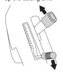
4 Release the clip on the front hood and lift off the fender.
