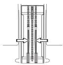
If necessary, the wires can be adjusted by tightening the adjuster nuts on each side of the steering collar. Do not over tighten the cables; they should only be drawn in towards the steering collar.
