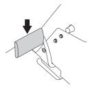
2 Carefully press down one of the pedals until the required speed is obtained. Pedal (1) is used to drive forwards, and pedal (2) to drive backwards.
