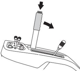
The lever can also be used to temporarily regulate the cutting height, e.g. for a small mound in the lawn.
