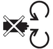
Rotary blades Keep hands and feet away from under the hood when the engine is running
