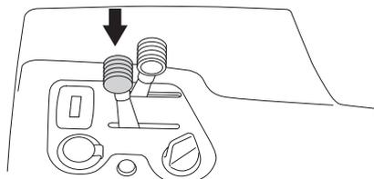
To increase or reduce the engine speed the control is moved backwards or forwards.
