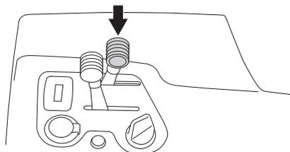
For cold starting the lever is moved backwards to its end position.
