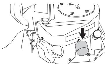
Lightly lubricate the rubber seal on the new oil filter using new oil. Fit the oil filter by turning clockwise. Turn by hand until the rubber seal is seated. Now tighten a further half turn.
