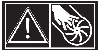
Do not place hands near rotating parts. Keep clear of the discharge opening at all times.
