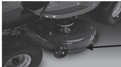
Stamped Deck Shell below, NOT reinforced
