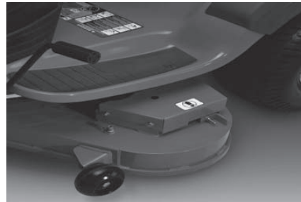
Fabricated Deck Shell Example Below
