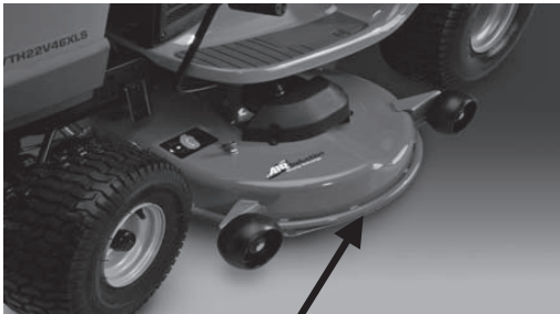
Armor Protected Stamped Deck Shell Example Below
