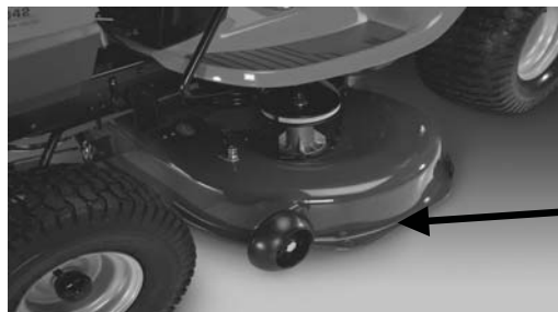
Stamped Deck Shell below, NOT reinforced
