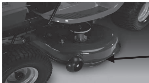
Stamped Deck Shell below, NOT reinforced
