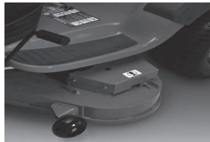
Fabricated Deck Shell Example Below
