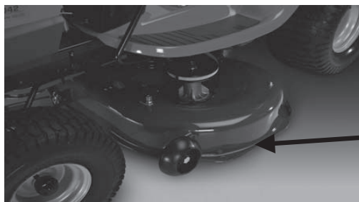
Stamped Deck Shell below, NOT reinforced
